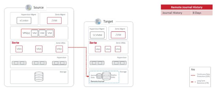
The disaster reference architecture depicted in figure 1 shows a set of proven practices for setting up the platform where a single remote target is being used as the recovery site.
